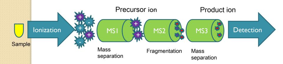
molecules determined based upon their mass-to charge(m/z)ratio
