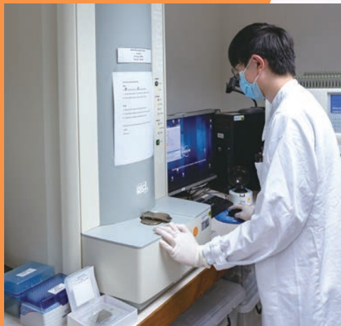
質譜儀可在數分鐘內鑑定細菌、真菌等微生物。MALDI-TOF mass spectrometry can provide rapid identification of microorganisms.
