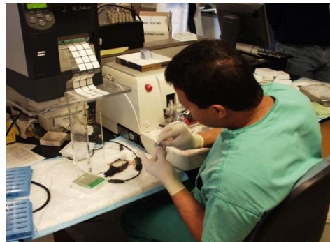
Bar Coded StainerShield Labels are Printed On-Demand at Cutting Station With Data Directly from LIS
